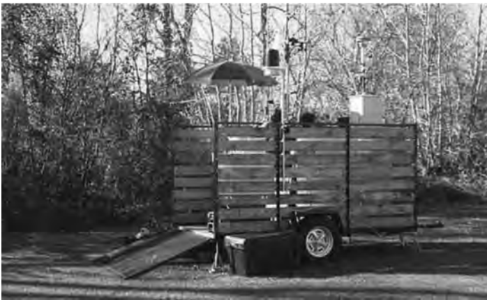
FIGURE 3.10 (See color insert.) Monitoring trailer used to house equipment for measuring hourly pollution levels in 16 neighborhoods in eastern North Carolina. (Courtesy of Denzler, B., University of North Carolina.)
